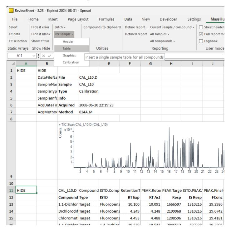
Adjust the width of columns C and E Double click between the header cell C and D, and between E and F
