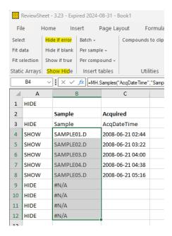
Column A cells contain a formula that return HIDE if a B column cell contains an error. In User mode, the rows with the HIDE will be hidden. The sheet is now independent of the number of samples in the batch.
