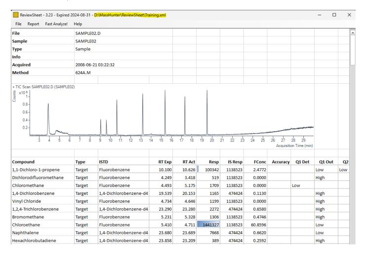
The rows and columns started with HIDE, are hidden Select another sample in MassHunter, the values are updated on the sheet Select an cell related to a different compound on the sheet, MassHunter navigates to that compound Perform a manual integration in MassHunter, the sheets shows the new response
